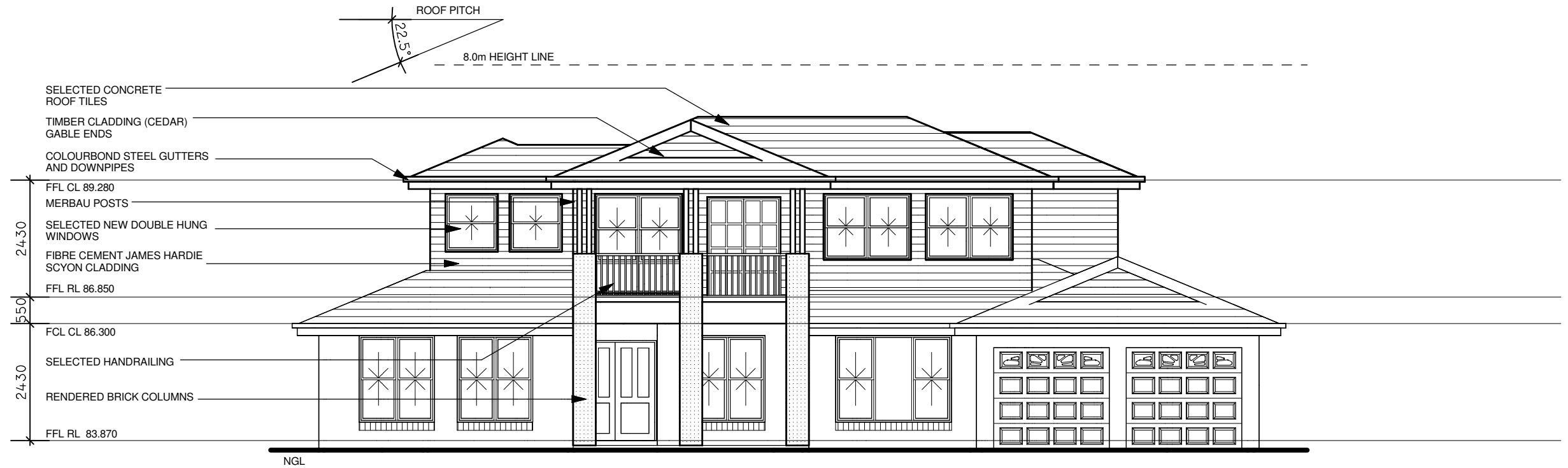
FRONT (NORTH) ELEVATION
